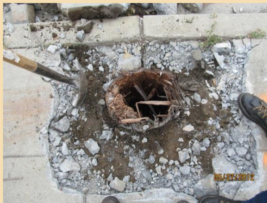
After extraction showing below ground deterioration
